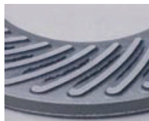
Casting without ANTRAPEX® can cause finning and veining.
